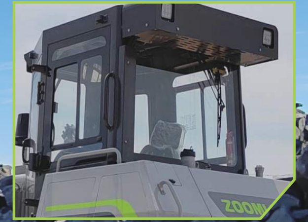
The top-mounted, high-powered air conditioner 顶置大功率空调
