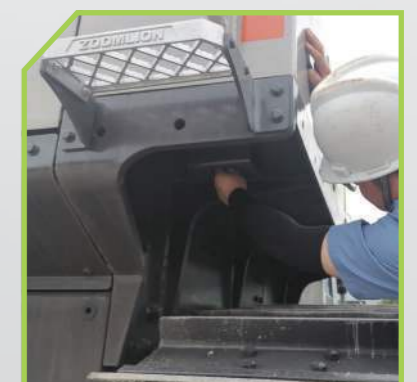
Oil tank draining 工作油箱放油
