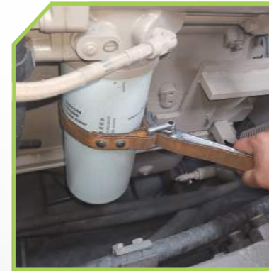
Oil filter maintenance 机油滤更换
