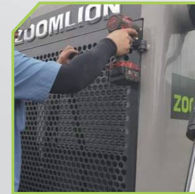
Radiator maintenance 散热器清扫
